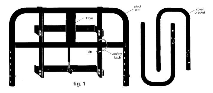
Position Cover Caddy centered side to side on spa cabinet (on side of spa with 3' clearance). Pivot arm must be even with top rim of spa. Use the 8 wood screws provided when mounting Cover Caddy through the 8 holes on the 2 support bars. MAKE SURE YOU ARE MOUNTING TO SUPPORT BEAMS (under outside cabinet). IF you cannot locate support beams or none are available to mount to,mount (2) 2x2 wood sticks to spa cabinet first,then mount Cover Caddy to 2x2s (fig.3).
