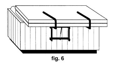
\*Note:If Cover Caddy is not opening or closing properly (too fast or too slow),the shock on the Cover Caddy can be adjusted to another hole on the "T bar". For a heavier spa cover, move to a hole closer to the spa cabinet. For a lighter spa cover, move the hole farther out. The shock comes installed in the proper hole for an average weight spa cover.
